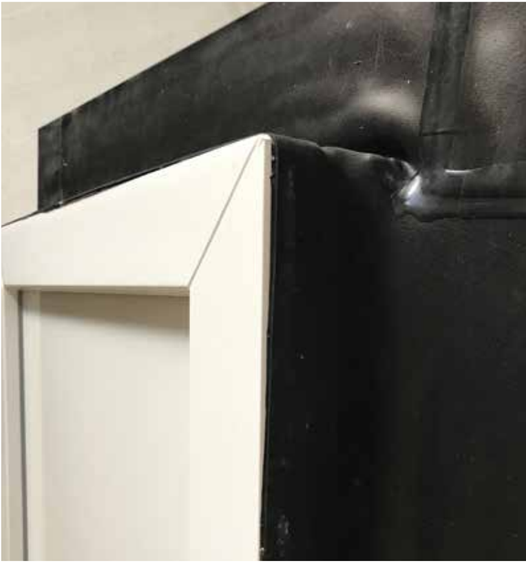
EPDM Window Frame test set-up at the University of Ghent
